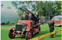
The Museum of Fire put on demonstrations of some of their vintage fire trucks. Here we have a 1929 Dennis truck with 4 cylinder petrol engine which drove the pump. The firefighters are dressed in period uniform. The brass helmets worn by the fire fighters were still in use in 1969, and a lot of time was used polishing them.
